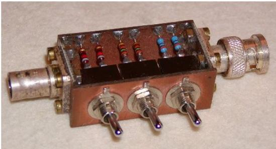
Example of a home-made switchable attenuator
