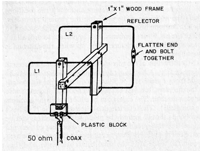
—Mechanical details of a 2-element quad for 144 MHz. The driven element, L1, is one wavelength long; reflector L2 is 5% longer. With the transmission line connected as shown here, the resulting radiation is horizontally polarized. Cuts of elements of this antenna are spaced 16 to 19 inches apart. The example shown may be fed directly with 52-Ω coax.
