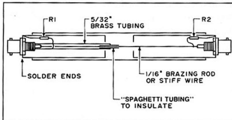
Figure 4. The final assembly of the attenuator.
