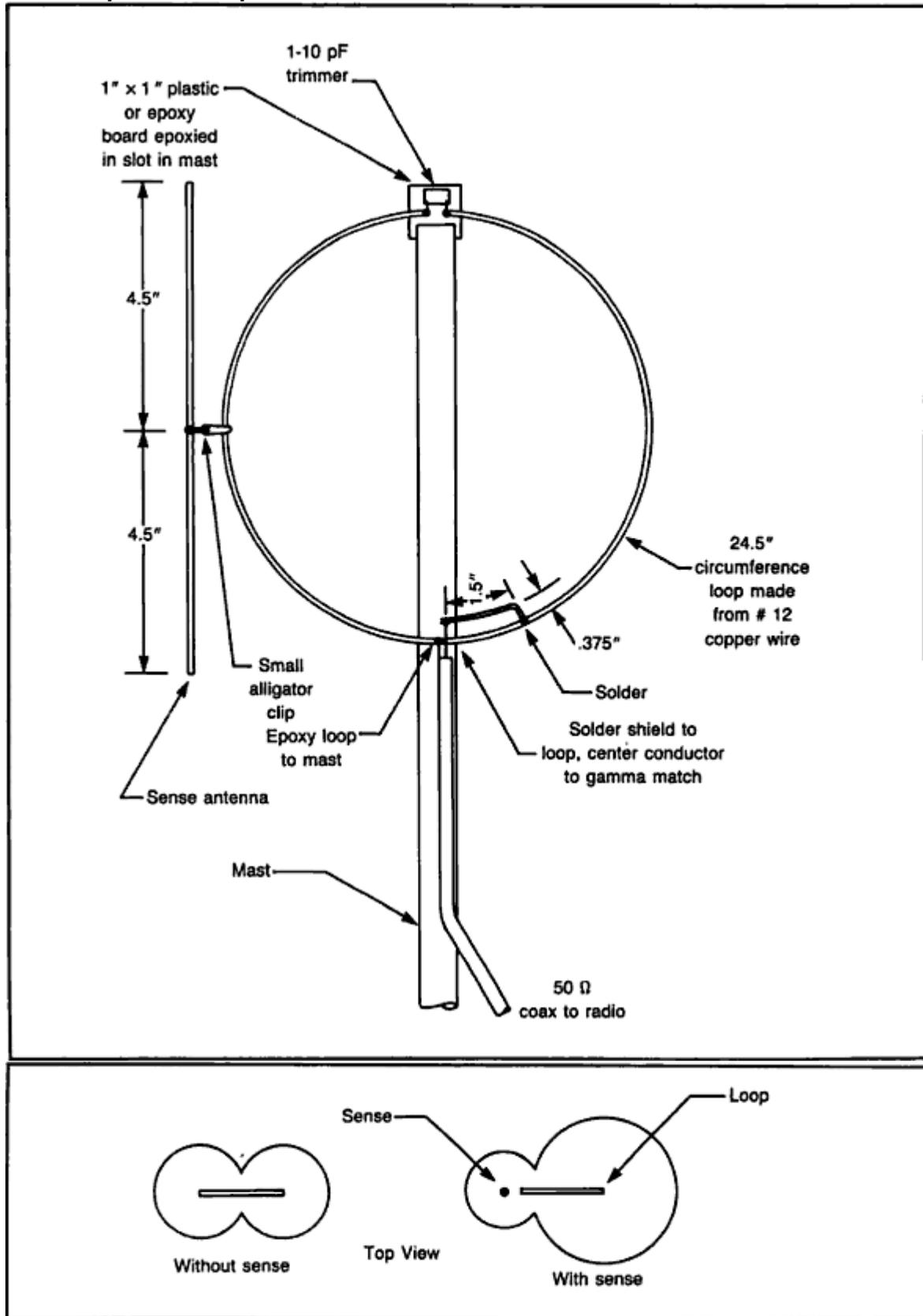
Antenna pattern without (left) and with (right) clip-on sense element. Mount on a broomstick mast. Use the nulls to determine the direction, attach the sense element and find the signal peak to determine which null points to the correct bearing.
