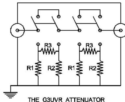
If accuracy is not important, substitute standard resistor values.
