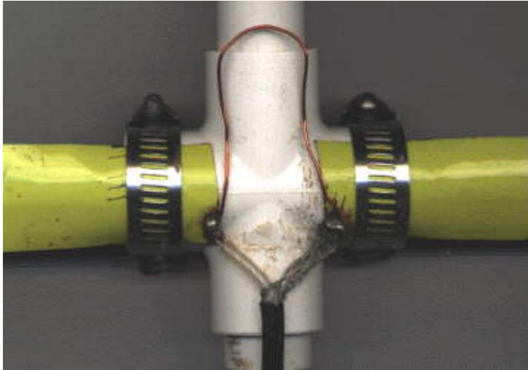
Close-Up view of RDF beam showing construction details and the "hairpin match" using a 5 inch length of 14 to 18 AWG solid insulated wire (1/4 inch bared for soldering at each end) connected across the feed points of the driven element (make the "U" about  $\frac{3}{4}$  inch across).
