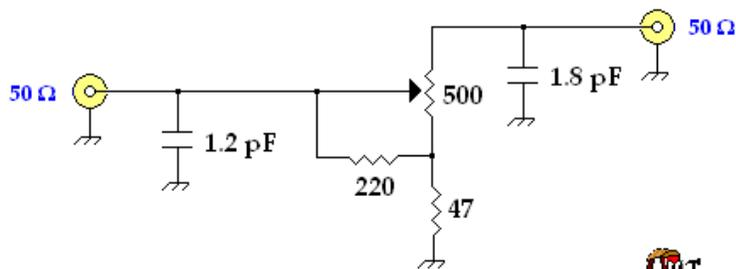
Simple attenuator produces about 20 db of attenuation.
