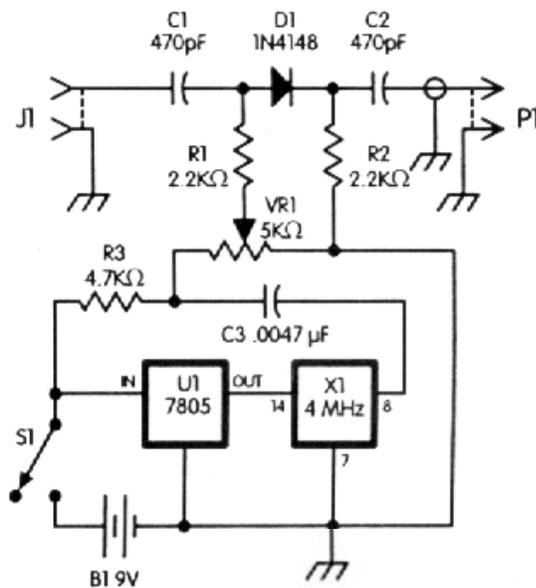
Example of an Offset Attenuator and the circuit diagram. The complete construction plans can be found at: <http://homingin.com/joek0ov/offatten.html>
