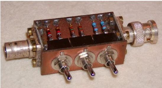
Example of a home-made switchable attenuator
