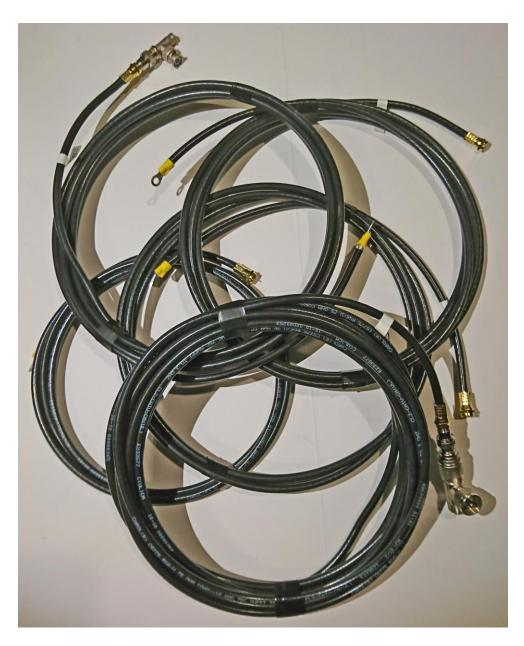
Set of 5 quarter-wave stubs for 10, 15, 17, 20 and 40m bands. I plan on also making one for the 80m band. These are compact and light-weight, and all fit into a small bag (wind some in diameters that can nest inside others). Don't forget to label each stub with the band it is for, as you make them. We will definitely be trying them out during the next Field Day with two 100W club stations; usually one is on SSB and the other on CW or a digital mode.
