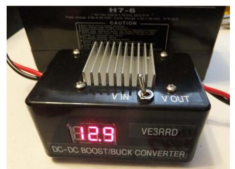
The finished converter allows me to use 6V, 12V or even 24V batteries to power my KX3
