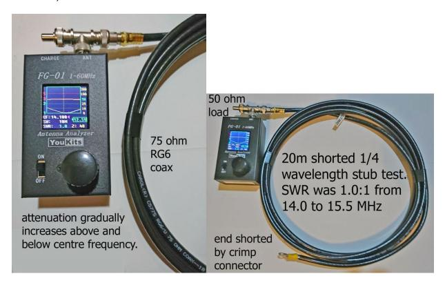
Everyone in our group has made a stub for each of the various HF bands they plan on using when we are operating together. I have found that these stubs even work well on the club TS-480SAT at 100W, and have also used them on my KXPA-100 PA when operating my KX3 at 100W. I used a UHF type T-connector on the transceiver/PA output and then used a UHF to BNC adapter to mate to the stubs.
