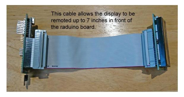
Unlike the BITX40v3 design; on the uBITX, the raduino board must remain plugged into the main board so that connections are kept as short as possible. If you are using a long enclosure and wish to mount the main board at the rear so that the two IRF510's can use the rear metal enclosure end as a heat-sink (using proper TO-220 transistor insulation kit), then you will need to move the LCD display forward while leaving the raduino attached to the main board.
