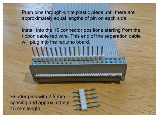
Since both connectors on the ribbon cable are female type, a "gender changer" is required at one end to plug into the raduino board.
