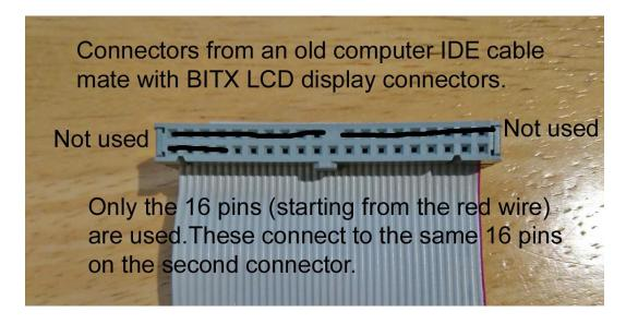
Use "Liquid Tape" or something to insulate the ends of the ribbon cable wires that were cut off so they can't accidently make contact with anything.
