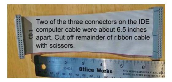
I used an ohmmeter to verify connectivity between the two connectors and found that the 20 pin row of one was wired to the same pins on the second connector.
